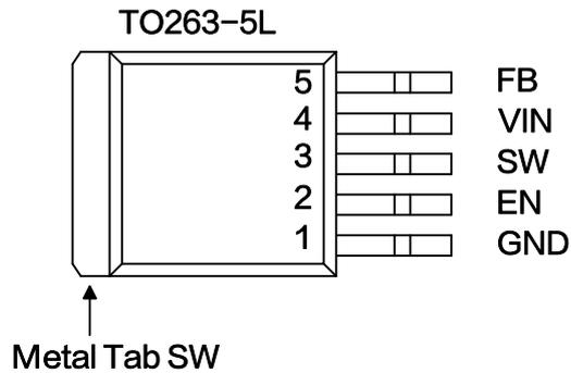
Figure2. Pin Configuration of XL6006 (Top View)
