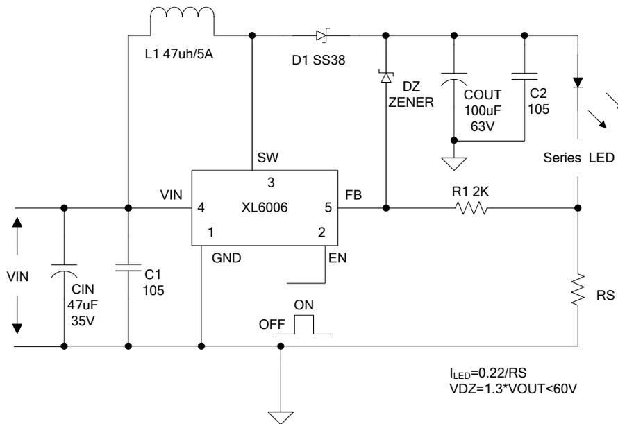
Figure11. XL6006 System Test Circuit (LED Open Protection)
