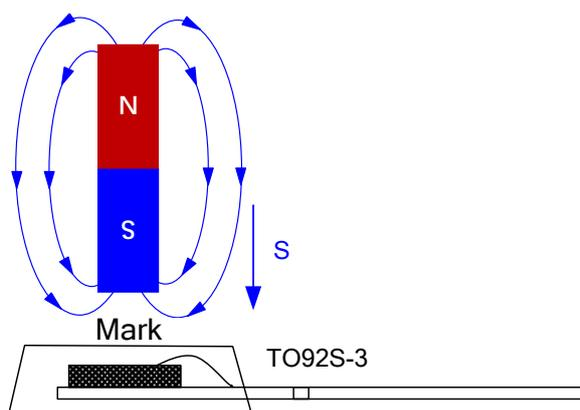
Figure4. Test Schematic of XL47T
